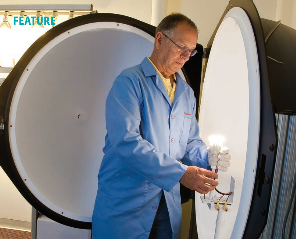
WINNERS CIRCLE Craig Limbert uses an integrating sphere to measure brightness and light color.
