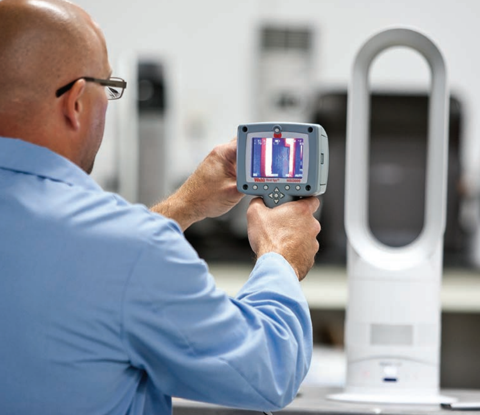
HEAT CHECK An infrared sensor measures surface temperatures on the top-scoring Dyson AM04.
